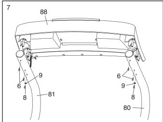
Carefully lower the Handrails (80, 81) to the floor. Center the Frame (59) between the Handrails. Tighten the four M10 x 58mm Bolts (4) and the two M10 x 110mm Bolts (3) (only one side is shown).
